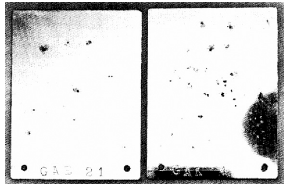
Figure 16 Increase in porosity of an electrodeposit caused by mechanical polishing. Left, 7.5 mm unpolished coating; right, polished with lime finishing compound. The average thickness removed by abrasion was 0.1 mm.
