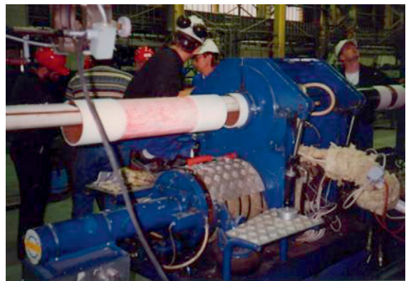
Figure 9 Injection molded polypropylene field joint coating application to pipe test pieces.
