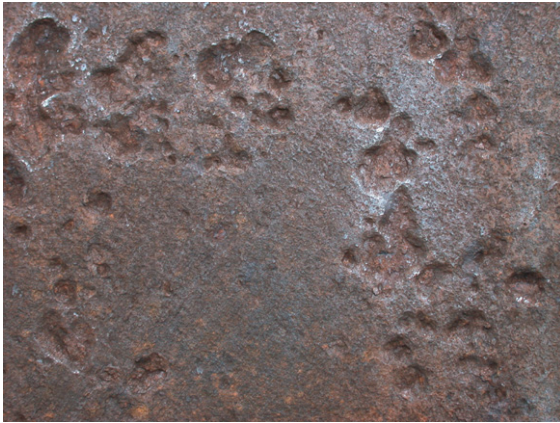
Figure 21 MIC pitting in an iron sulfide film, morphology of micropits within larger pits. Reproduced from Stott, J. D. F. Microbial Environments . In Corrosion ; Elsevier: London, 2009; Vol. 2.
