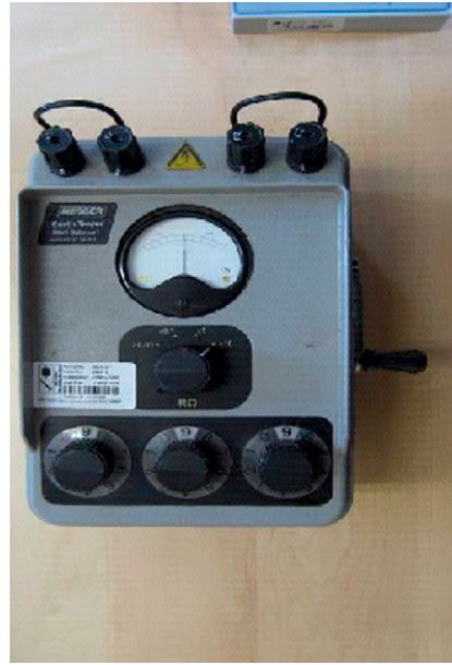
(b) 4 Pin Earth Resistivity Meter using a hand cranked AC generator. More modern devices use battery/electronic AC circuits but this device remains one of the most sensitive
