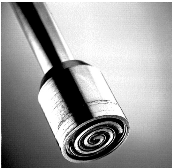
Figure 2 Electrical resistance (ER) probe – spiral wide tip (Courtesy Cormon Ltd).
