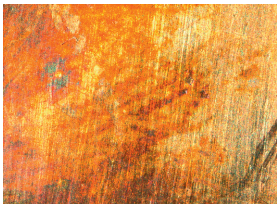
Figure 6 The influence of a fingerprint on the pattern of sulfur tarnishing on this silver surface is clearly visible. A protective coating on the surface would have prevented this.
