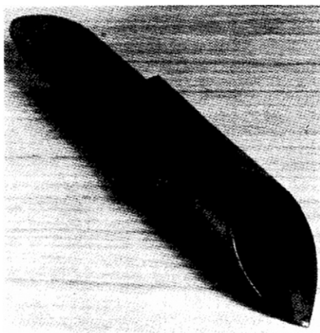
Figure 12 An electrodeposit showing unusually high compressive stress. A 150 × 150 mm copper sheet was insulated with lacquer on one side and electroplated with Sn-35 Ni alloy. The high compressive stress has caused the sheet, originally flat, to coil in the manner shown, with the electrodeposit outside.
