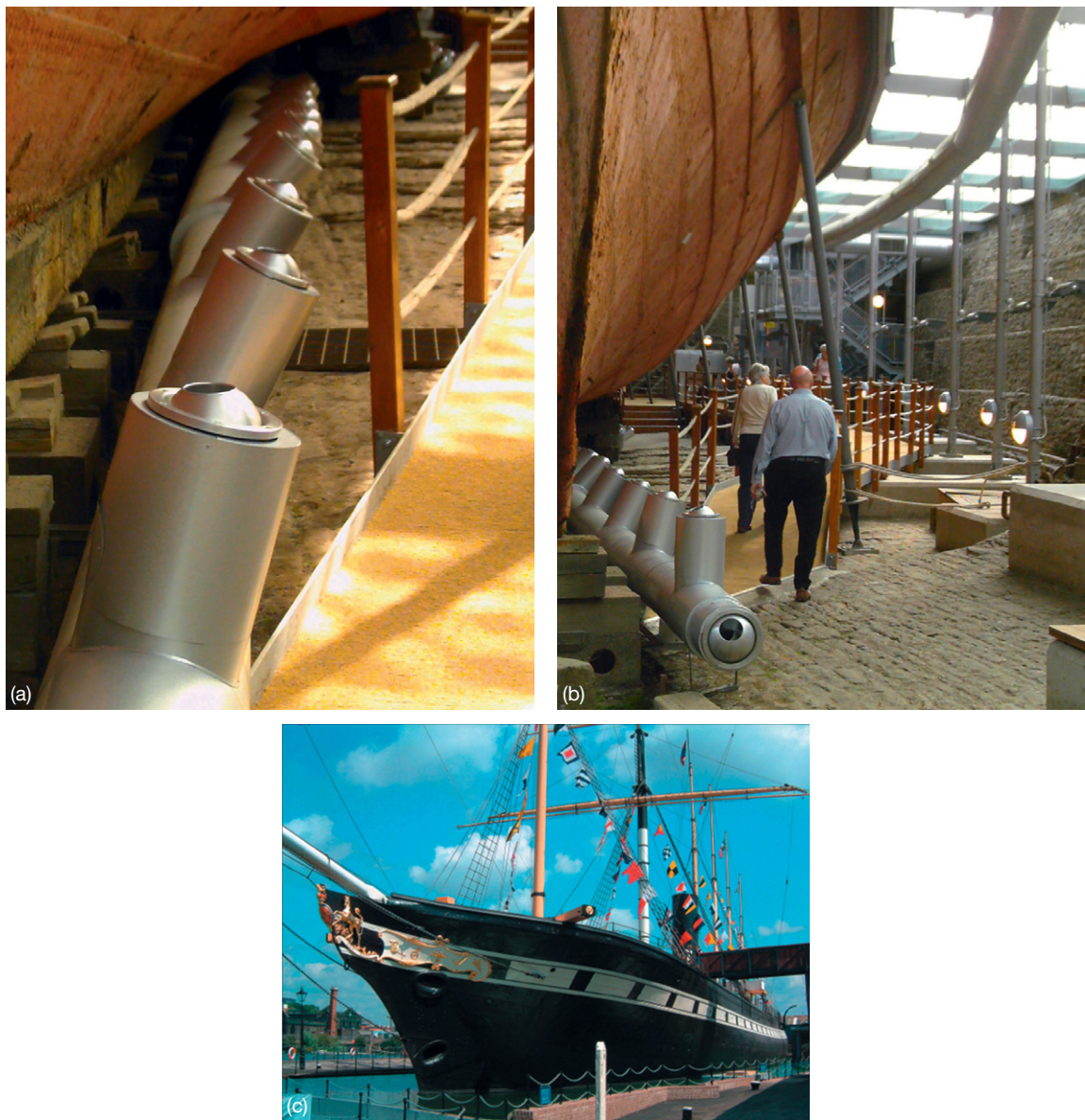
Figure 8 Brunel's iconic SS Great Britain was the first ocean going screw driven iron hulled passenger liner and is now preserved by a mechanical desiccation system that maintains relative humidity to 20% and allows visitors to walk around the hull. Reproduced from Watkinson, D.; Tanner, M.; Turner, R.; Lewis, M. The Conservator 2005 , 29, 73–86. 25
