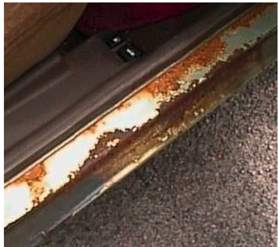
Figure 3 Corrosion along a door sill.
