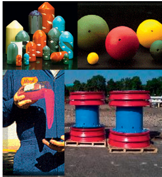
Figure 8 Gel pigs, spheres, and product separating pigs employed to trap a slug of treating chemical.
