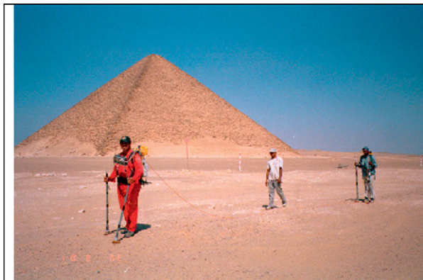
(a) Combined CIPS and DCVG survey (courtesy Corrosion Control Services Ltd.)
