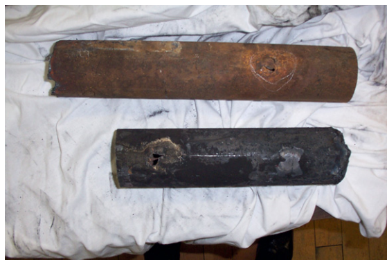
Photo 6 MIC on a sectioned pipe.
