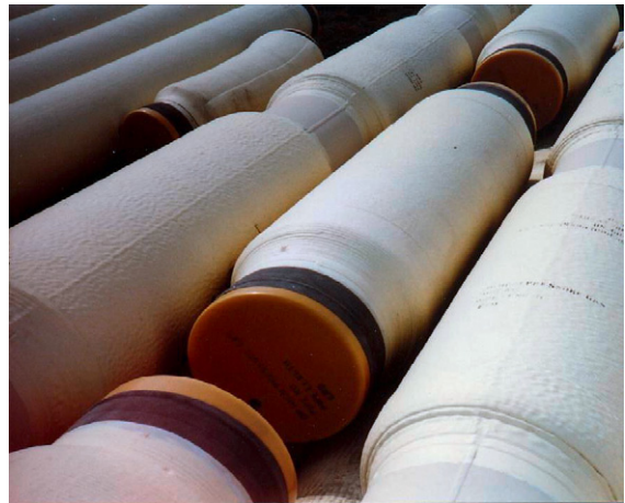
Figure 13 Thermally insulated line pipe awaiting pipeline construction.
