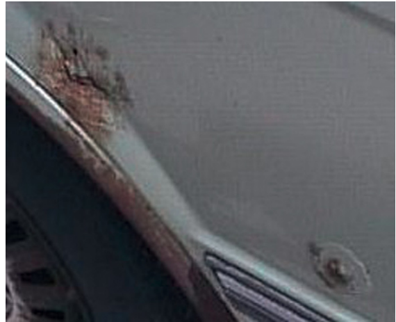
Figure 1 Incipient panel perforation.
