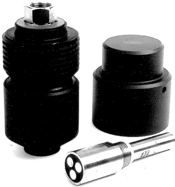
Figure 7 Linear polarization resistance (LPR) electrochemical probe and 'access fitting' (Courtesy Cormon Ltd).
