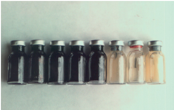
Figure 22 Serial dilution test for SRB, five dilutions contain bacteria indicating a heavy infestation.
