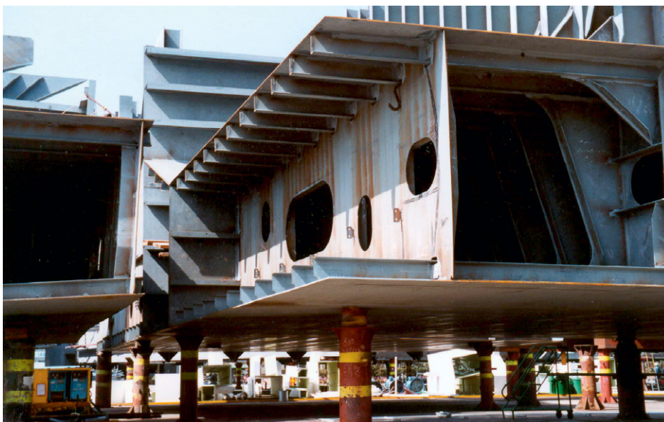
Figure 6 Block section from a VLCC.
