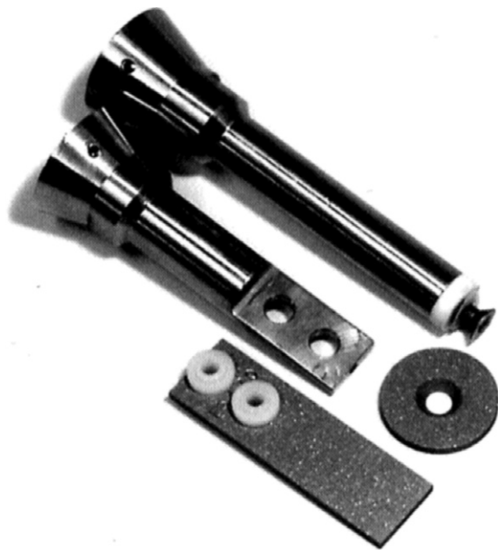
Figure 1 Corrosion coupon holders and corrosion coupons (Courtesy Cormon Ltd).
